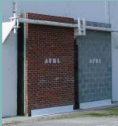
Masonry walls in test frame just prior to loading
